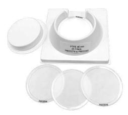
GVS Life Sciences PM 2.5 PTFE Membrane is a high-purity, thin membrane for PM 2.5 ambient air monitoring. Each membrane is sequentially numbered with a chemically resistant polypropylene support ring. The low tare mass allows for accurate gravimetric determinations. No glues or adhesives are used in making the membranes and its stable design eliminates curling, keeping the membrane flat allowing for robot use.
