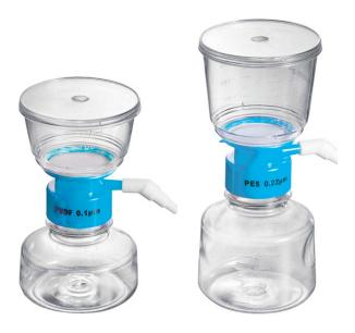
GVS Vacuum Filters are very useful in large volume samples separation and purification.
